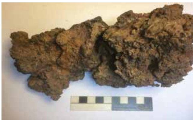
App. B.1 Plate 1: Three re-fitting pieces of vitrified clay melted in front of the tuyere hole of an iron smithing (re-used saltern) hearth. Context 909, Saltern 6
